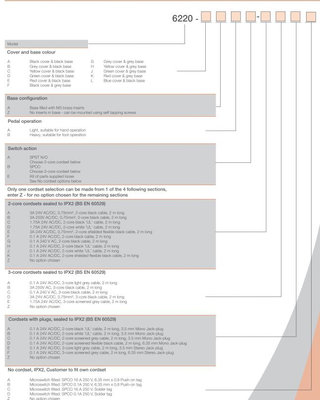
Note: The cordset rating must exceed the maximum control circuit rating. Options B & D are low power switches and must only be used in applications where suitably designed constraints are met.
