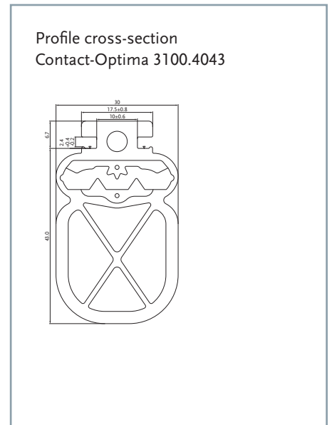
For dimensions without tolerance particulars, tolerance-free dimensions as per DIN ISO 3302-1 E2 shall apply.
